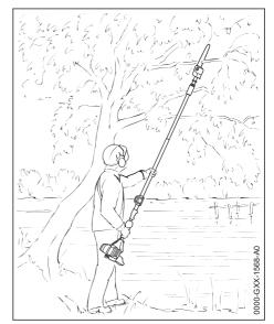
The machine's long reach makes it possible to prune branches that are overhanging obstacles, such as rivers or lakes. The tool angle in this case depends on the position of the branch.
