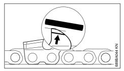
File the top of the depth gauge parallel to the stamped service marking (see arrow) – but do not lower the highest point of the depth gauge in this process.
