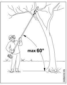
Hold the power tool at an angle. Do not stand directly underneath the limb being cut. Do not exceed an angle of  $60^{\circ}$  from the horizontal. Watch for falling wood.
