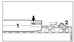
Place a filing gauge (1) that matches the chain pitch on the chain and press it against the cutter – if the depth gauge projects from the filing gauge, the depth gauge has to be lowered.
