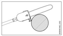
When performing the separating cut, position the bar against the branch near the hook. This will prevent the power tool from making jolting movements when you start the separating cut. Always cut with a correctly sharpened, properly tensioned saw chain – the depth gauge setting must not be too large.
