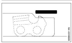
File down the depth gauge until it is level with the filing gauge.
