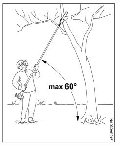
The shaft should always be held at an angle of  $60^{\circ}$  or less.
