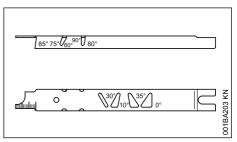
Use a STIHL filing gauge (special accessory, see table "Sharpening Tools"). This is a universal tool for checking the filing and side plate angles, depth gauge setting, cutter length and groove depth. It also cleans the guide bar groove and oil inlet holes.
