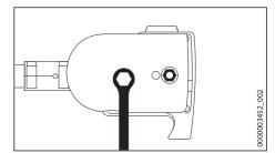
Unscrew the nut and remove the cover
