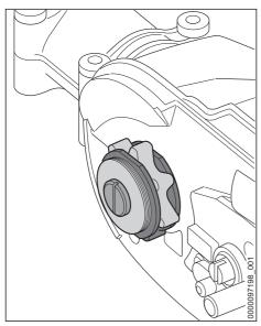
The chain sprocket is driven via a friction clutch. Have the chain sprocket replaced by an authorized dealer.
