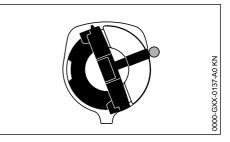
Markings on fuel cap and oil tank must align
