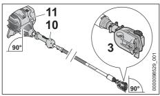
Align the housing (11) (with the manual fuel pump facing up), the control handle (with the stop switch facing up) and the transmission (3) (with the oil tank cap facing up) as shown
