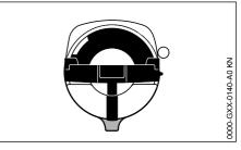
Then the markings on fuel cap and oil tank will align
