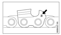
The chain pitch (a) is marked on the depth gauge end of each cutter.
