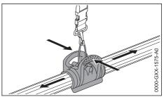
Squeeze the clip (carrying ring) together to move it up or down the shaft
