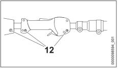
Tighten down the screws (12) firmly
