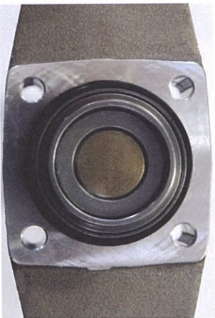
Figure 4 Bottom assembly top view CHPD52
